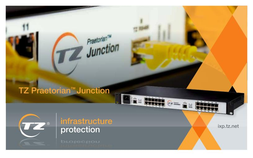
The TZ Praetorian Junction interprets relay output signals from building access control systems and converts them into RS485 serial data signals to communicate with TZ locking devices and also to supervise door position sensors, detect intrusions and override key door opening which are reported back to the building access control system through its associated relay inputs.
